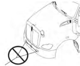
3. NEVER USE SINGLE CHAIN OR CABLE LOOPED THROUGH TOW DEVICES
