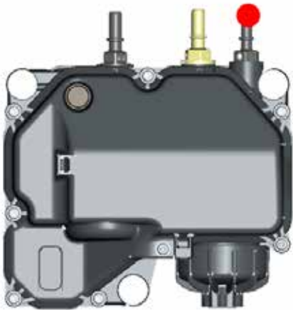
FIGURE 5-1: Measurement Location of DEF Supply Module (Pump)
