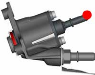
FIGURE 5-2: Measurement Location of DEF Dosing Module (Injector)
