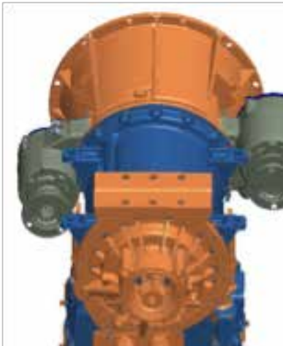
FIGURE 4-5. Allison 3000 Series Transmission PTO Locations
