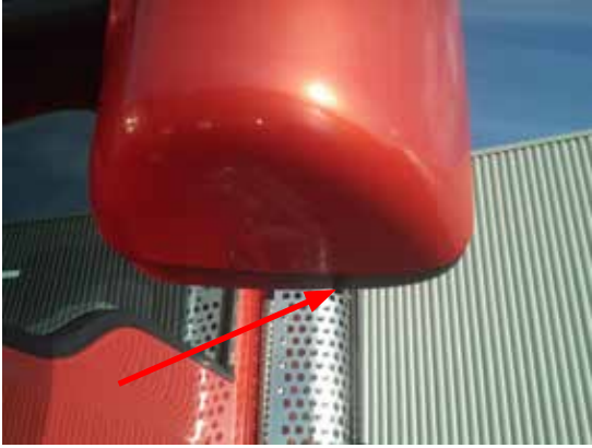
FIGURE 2-3: Aerodynamic Mirror OAT Sensor Location
