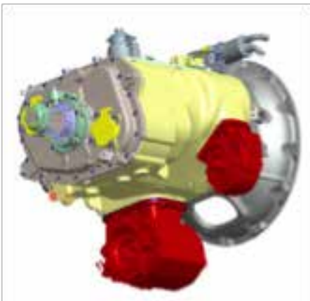
FIGURE 4-2. Heavy Duty Manual Transmission PTOs
