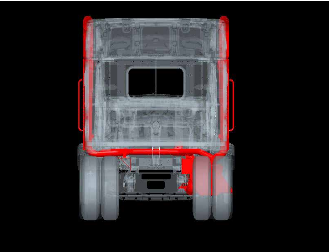
FIGURE 5-48: Rear View of Right Hand Under DPF/SCR with Dual Back of Sleeper Tailpipes (52" Sleeper)
