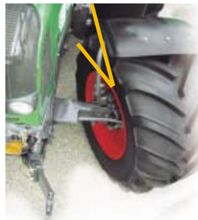
Mudguards on the front wheels can be swung out to maximise steering angle.
