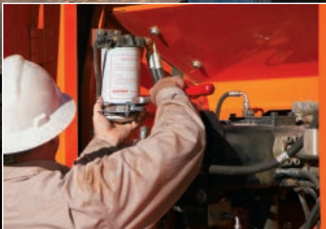
Ground level access to all filters
