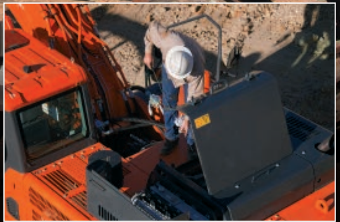
Easy access to regular inspection points
