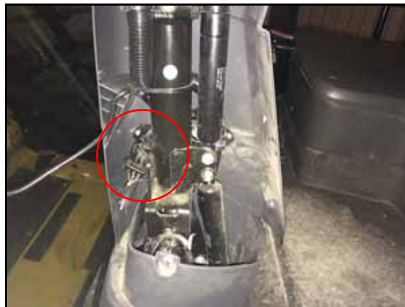
FIGURE 6. Steering Wheel Sensor and Connections
