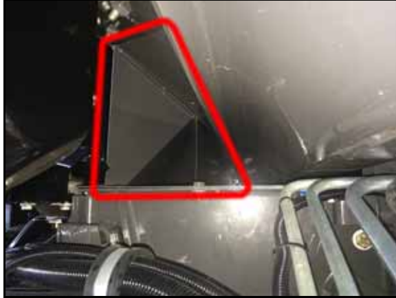
FIGURE 7. Access Area for Routing Valve Harness
