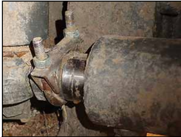
FIGURE 8. Small Muffler Clamp Installed
