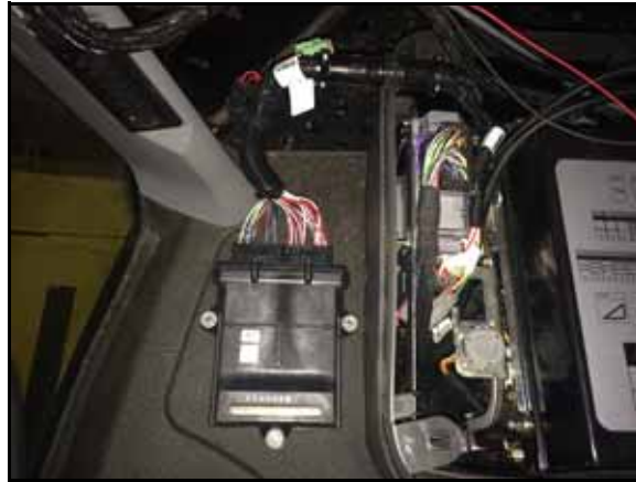
FIGURE 5. Node Harness Installed on SmarTrax Node
