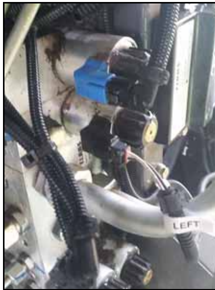
FIGURE 13. LEFT Valve Harness Connector Installed
