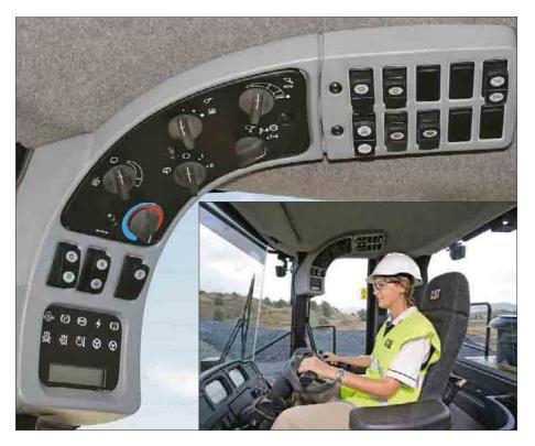
**Controls.** The main control panel on the 980H is located high on the right ROPS post – keeping everything within reach of the operator while maintaining visibility to the ground. Keeping all switches and controls conveniently placed allows better operator efficiency and improved productivity, while minimizing operator fatigue.
