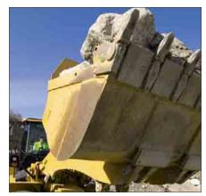
**Automatic Kick-Outs.** The standard programmable automatic kick-outs provide flexibility and productivity for precise load and dump target heights. Tilt, lift and return-to-dig kickouts are set by positioning the bucket or work tool and setting a rocker switch in the cab.
