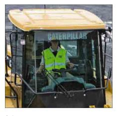
**Cab.** The entire operator station can be removed in about 45 minutes and is easy to re-attach. Quick disconnects are used so no wires need to be cut and no refrigerant is lost.
