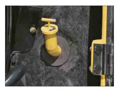
With the hood closed, quick checks of engine oil level and the coolant sight gauge can be completed through the side service doors.
