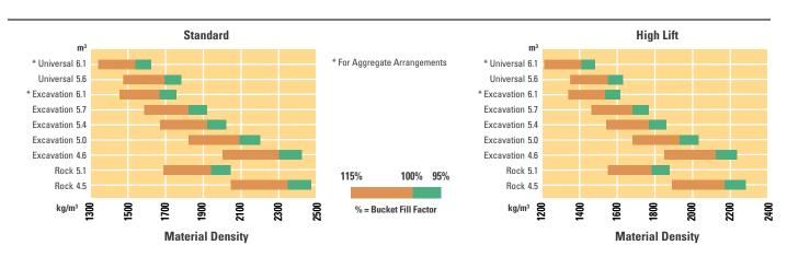
In accordance with SAE J818, these data consider the bucket load to be equal to half of the static tipping load at full turn.
