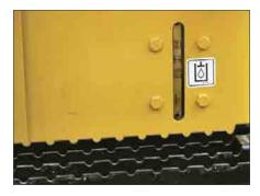
**Sight Gauges.** Well-protected, yet easily visible sight gauges for the transmission oil, hydraulic oil and engine coolant allow easy daily checks while reducing the risk of contaminants entering the systems.
