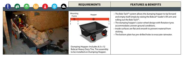
**Description:** Park it, load it and dump it. This attachment mounts as easily as a bucket on your loader, and can go wherever your loader goes. Empties fast and easy, just raise the loader arms and dump. Flat, smooth interior surfaces prevent materials from sticking.
