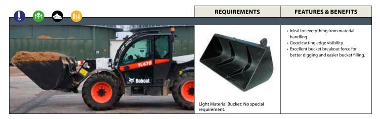
**Description:** The large capacity of the Light material bucket is designed for loading and handling various light materials such as mulch, snow and grain. These buckets have high backs and straight sides to penetrate piles with ease.
