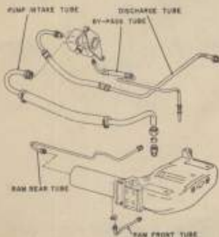
Fig. 13—Drawing showing the positions of the various power steering tubes used on all D-15 diesel tractors and D-17 diesel models prior to tractor Serial No. D17-38964.
