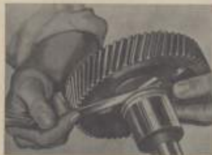
Fig. 46—To check the diesel engine camshaft end play, insert a feeler gage as shown between shaft journal and the thrust plate. The amount of end play is equal to the thickness of the maximum size feeler gage that can be inserted.
