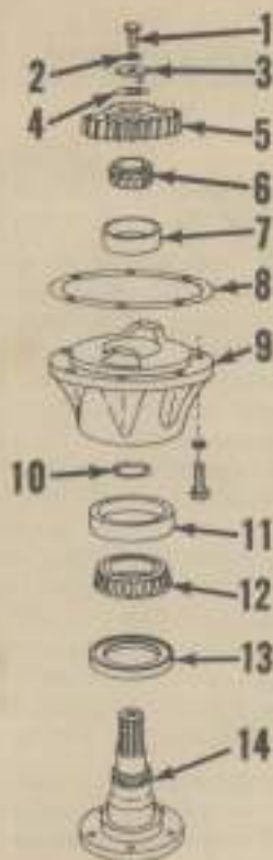
Fig. 24—On single front wheel tricycle models, above parts are used in steering gear instead of items 53 through 62 shown in Fig. 23. Mark on hub of sector gear (5) must be aligned with punch mark on top of sector shaft (14).
