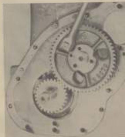
Fig. 45 — Removing the camshaft thrust plate retaining cap screws. (Although a WD45 diesel engine is shown the method is the same for D-15 and D-17 diesel models.)
