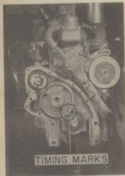
Fig. 43—D-14 and D-15 non-diesel timing marks on camshaft gear and crankshaft gear. The governor and distributor drive gear, also shown, may be meshed in any position; ignition timing being made at distributor. Timing marks for D-17 non-diesel engines are similar.
